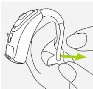
ⓘ Please try to avoid gripping the tube to remove the CROS device.
