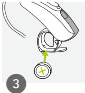
Place battery in the battery door with the "+" symbol facing upwards.
